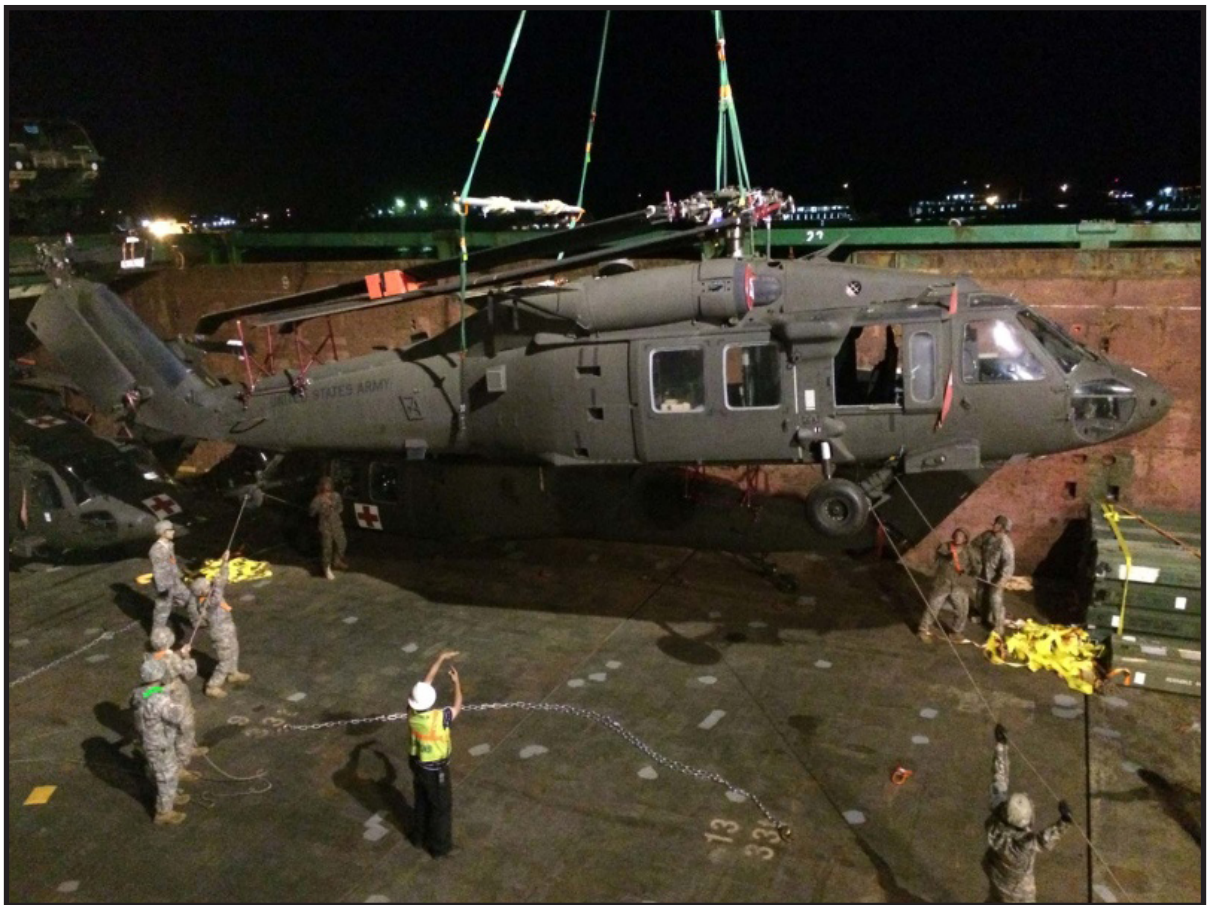
Figure 20.2 A helicopter is lifted out of a cargo ship on 23 August 2014, at Banyuwangi Port for delivery to the Garuda Shield exercise. The sling holding the helicopter was a new design for Pacific Pathways, and unlike old versions the new slings can be used indefinitely. Photo courtesy of the US Army.
